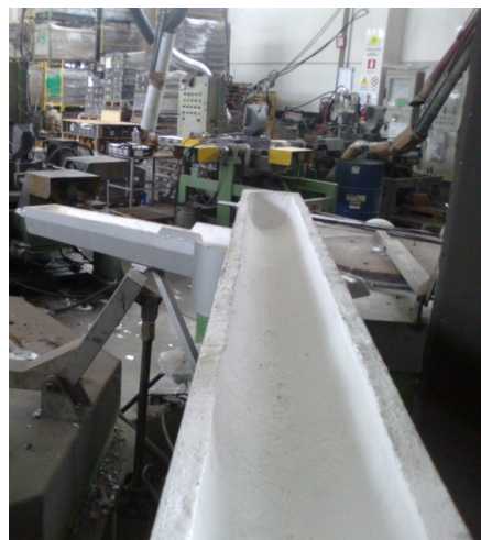
Pic 1: ISOPLAST E-AL application by hand on casting runner
