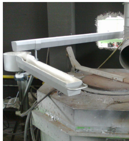
Pic 2: ISOPLAST E-AL application by hand on casting runner
