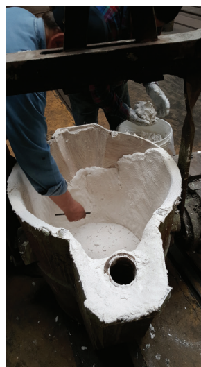
Pic 2: ISOPLAST HT application by hand
