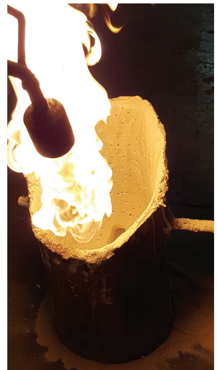
Pic 4: drying of ISOPLAST HT with 40 mm thickness
