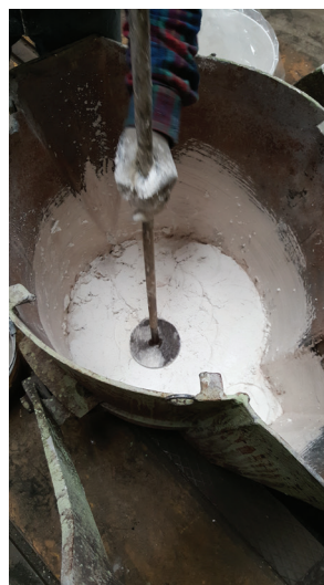
Pic 1: ISOPLAST HT application by slow ramming
