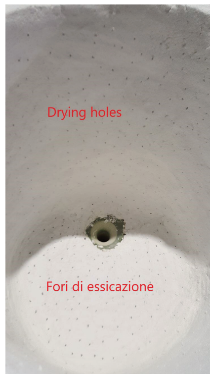
Pic 4: drying holes in ISOPLAST HT
