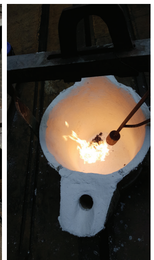
Pic 1: ISOPLAST HT drying with burner
