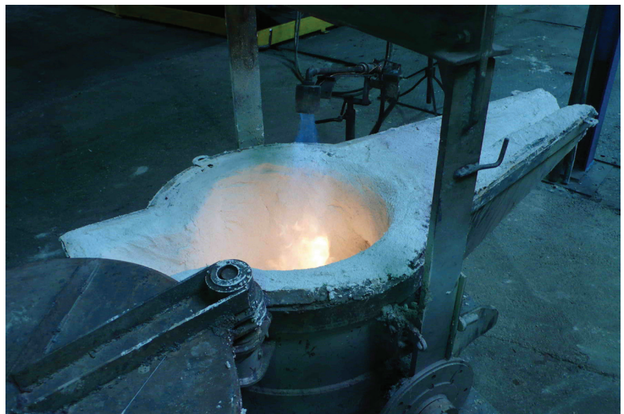
Pic 4: drying with burner
