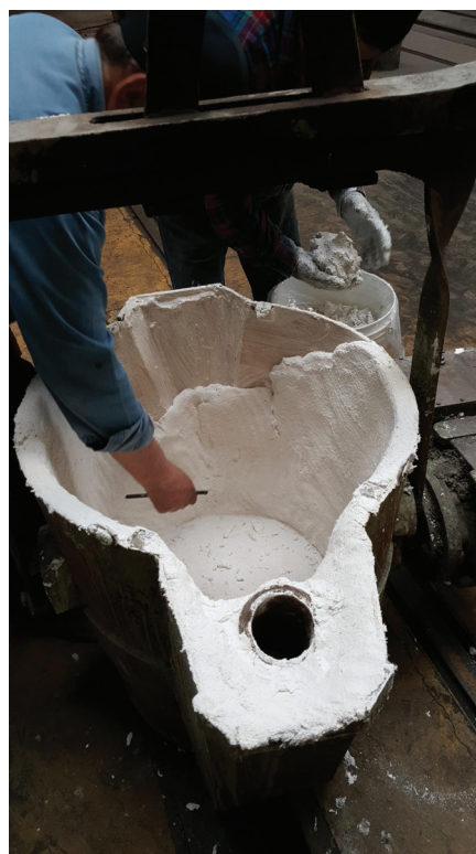
Pic 1: ISOTOP 2000 application by hand on pig-iron ladle
